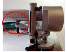
VTA (Vertical Tracking Angle) Adjustment It is assumed you have got the spindle at roughly the right height (see Page B Step 4) Twist the knurled dial anticlockwise to wind the 'fork' down till it touches the mounting plate.
