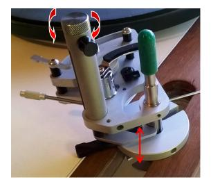
Step 2; The main spindle has two separate locking mechanisms
