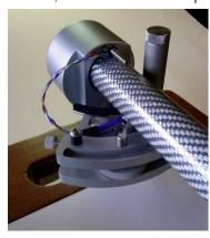
**Step 4**; **Overhang setup.** A) Swing the protractor and arm round so the stylus is above the arc XY **NOTE**; **To avoid damage to the stylus, do not let it touch the protractor (hold slightly above)**
