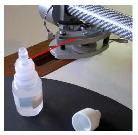
Step 2; Engaging the Vibration Shunt. With the arm in place, raise the trough by turning the knurled dial clockwise. Raise it till the threaded rod on the underside of the arm is just in the silicone. Listen!
