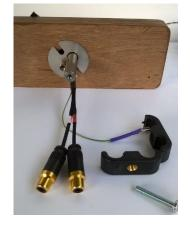
Step 3; Use the supplied 4mm Bolt to secure the plugs to the shaft.
