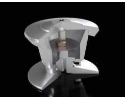
The *base of the clamp* is of a *separate piece* connected to the main chassis with a screw-locked cap which is decoupled by a *ceramic ball* at the apex of the pin. Thus, the base is free to *rotate independently*.
