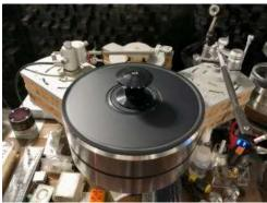
He believes that any record player, the *turntable* of whatever design is a source of (*internal*) *vibration* (from the motor, revolving platter, bearing, etc), that inevitably transmit that vibration to the pick up transducer, the phono cartridge. Therefore, the more elaborate turntable designs always incorporate mechanical vibration elimination (/extinction as the term preferred by Nasotec) contraption(s), which ultimately the higher retail price.
