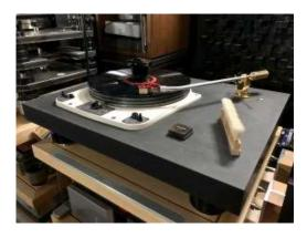
The vinyl records are cut using a *tangential cutting lathe* such as the *Neumann VMS80*. However, most playback of those vinyl records use the common pivot tonearm where mathematically **only two points** on the records that the stylus will be perpendicular to the grooves. Whereas at other points, it won't be able to track the grooves in the same manner as the record is cut using a tangential cutting lathe.
