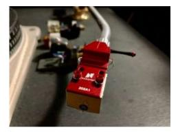
Given the circular grooves on a round record rotating at a certain fixed speed (33.3 / 45 / 78 rpm) mean *where the record is being tracked* require slightly *different angle at the <u>headshell</u> to track accurately*. The first track's or the start of the record's velocity is higher than the last track's or end of the record's. Therefore, slightly more angle or swinging at the headshell where the record is traveling with more friction or faster movement (eg; at the start of the record).
