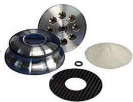
The VPI clamp has two damping rubber bands around the low circumference. The Silentor has a thin carbon fiber layer on the bottom where it contacts the LP label, which covers eight holes filled with crushed quartz for improved damping. A rubber O-ring fits over the spindle for additional damping. (It makes a cute little 'pop' sound when the clamp is lifted off.)
